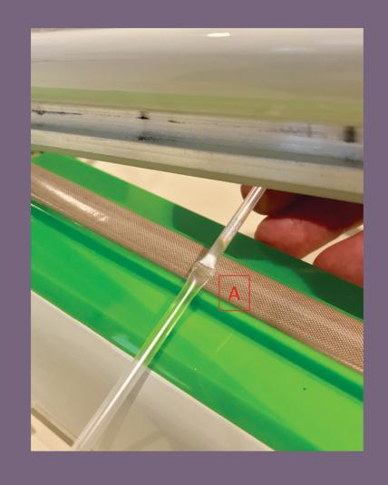
To prevent the wicking potential of the cotton-PVA plug in semen straws, we have added an inner weld seal (A) to our device system, as well as the weld seal on the end which secures our colorized label and weighted rod (B). The VTF tip is then inserted and sealed closed (C/D).
